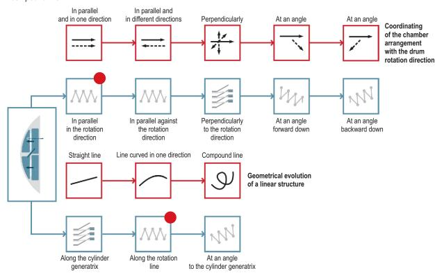
The Evolution Tree fragment for a real system – a solution supply device – will look as follows. The evolution pattern "Coordinating of the chamber arrangement with the drum rotation direction":
