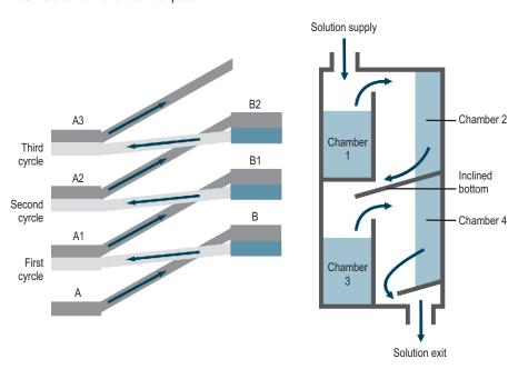
What can the structure of a device with a vertical arrangement of modules be like?
