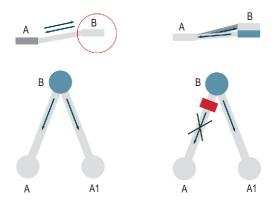
It is apparent that at fast rotation and due to the action of the centrifugal force, the liquid starts flowing into the second chamber and remains there until the rotation ceases. Then the liquid starts flowing through the inclined channels into the first and third chambers.
